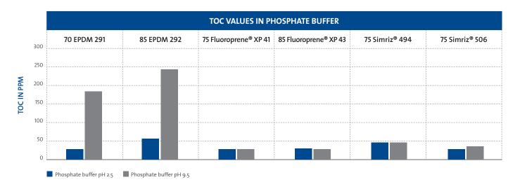
The diagram shows the TOC values of the tested materials compared to two black EPDM materials from Freudenberg.
